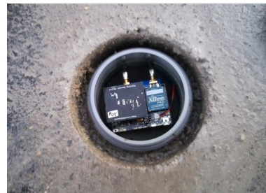
Wireless vehicle-presence sensor with 7 to 10 years of battery life http://embedded-computing.com/articles/sensor-enabled-nodes-support-the-iiot-for-smart-buildings-and-smart-transport/
