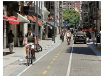
Buenos Aires, Argentina. A two-way cycle lane on a one-way street increases connectivity.
