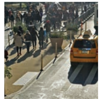
Planters and paint used to create an interim plaza.
