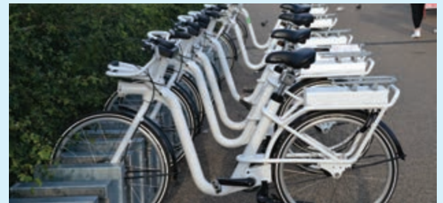
Copenhagen, Denmark. This share system provides pedal-assist e-bikes with built-in wayfinding screens.
