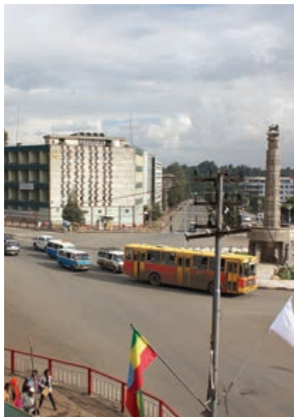
Addis Ababa, Ethiopia. A very wide traffic circle where the central space is inaccessible. Pedestrians have to cover very long distances in order to cross the street due to the wide diameter of the traffic circle. Sites like this present a great opportunity for redesign.
