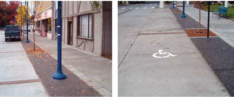
▲ Special paving treatments, landscaping, and other elements can be used to delineate spaces within the right-of-way
