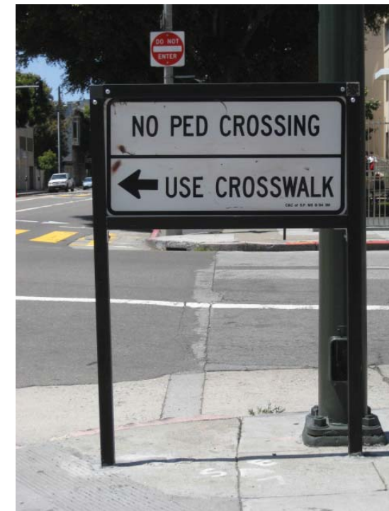
▲ Intersection leg closed to pedestrian crossing
