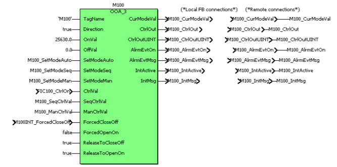
(*Device Interlocks for pump M100*)
