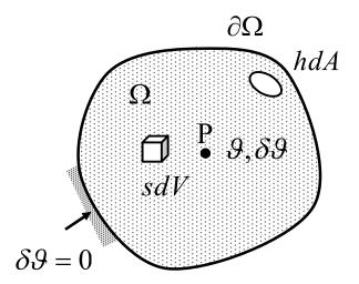
Finite element method is applied in the usual manner by considering temperature as the unknown. The physical dimensions  $[\delta P] = \text{Nm/(Ks)}$  and  $[\delta W] = \text{Nm}$  differ!
