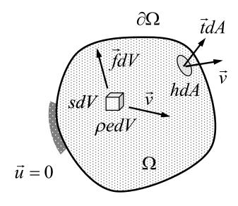
Constitutive equations of the form  $\vec{q}(\theta)$  and  $\vec{\sigma}(\vec{u},\theta)$  are needed for a closed equation system in terms of displacement and temperature.
