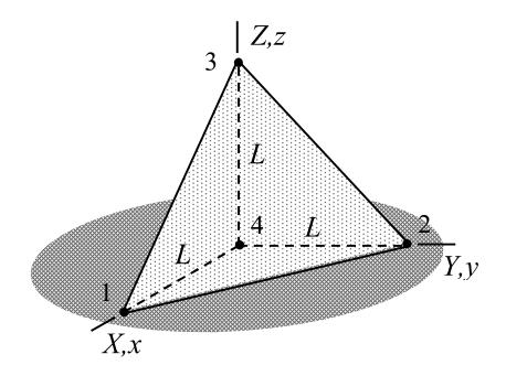
• Only the shape function  $N_3 = z/L$  of node 3 is needed as the other nodes are fixed. Approximations to the displacement components are
