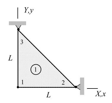
• The active degrees of freedom are  $u_{x1} = u_{X1}$  and  $u_{y1} = u_{Y1}$ . The linear shape functions  $N_1 = (L - x - y)/L$ ,  $N_2 = x/L$  and  $N_3 = y/L$  can be deduced from the figure. Therefore, approximations are
