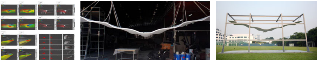
Figure 21. (Left) Solution space of synthesized designs using a hybrid computational fluid dynamics (CFD) and architectural design approach (Kajijima et al. 2013); (centre) production of the final prototype; (right) testing of the final design. The structure can passively reduce temperature at a bus stop by accelerating ambient winds, Courtesy of the SUTD-MIT International Design Centre.
