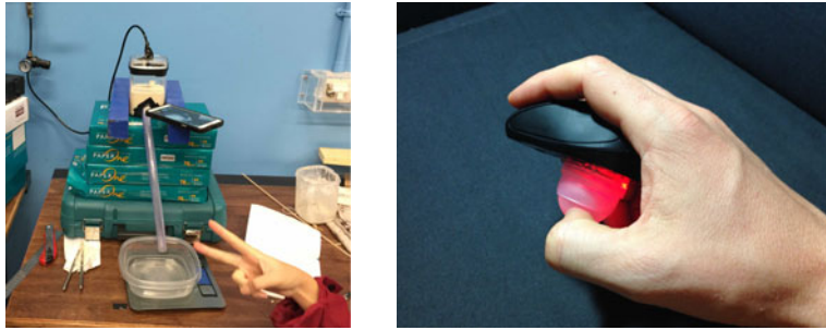
Figure 26. (Left) A simple configuration to test viscosity of a composite slurry using recycled storage container as a pressure vessel; (right) using rolling applicator as a modification to prototype a table-less mouse.
