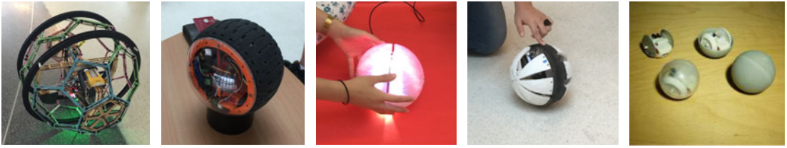
Figure 9. An example of competitively produced prototypes, from the 30.007 course at SUTD. (from left to right) A flying-rolling robot; rolling robot with enhanced traction wheel; rolling robot with active camouflage; rolling robot using exo-skeletal modular pendulums; integrated design for full project (semi-final design). These designs are part of a student design hackathon, which in turn is part of a larger university wide competitive project to develop advanced ISR robotics.
