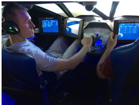
Figure 25. Haptic interface, in this case, a multi-functional display is simulated for a reusable launch vehicle with various interactive display mechanisms and controller feedback points. Courtesy Gilmour Space Technologies.
