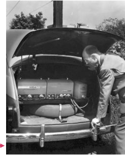
Bell System Motorola "Deluxe" line high band ( 150 MHz) "Urban" radiotelephone in 1948
