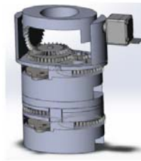
Figure 2 - The latest prototype of the two DoF (flexion/extension and rotation) wrist unit. The system turned out to be light though too long and consequently fragile.
