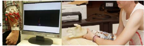
Figure 1 – LEFT: testing of the two DoF controller in the virtual reality through a set of multi-DoF tasks. RIGHT: testing of the system with the patient using a prototype wrist system, which seems to be too bulky for a prolonged use.
