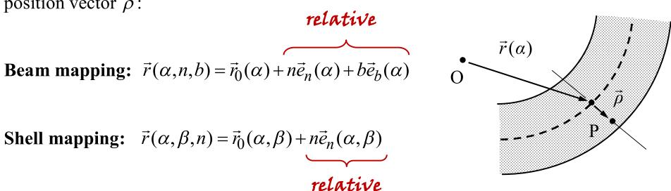
The mapping for the mid-curve or surface is used to define the basis vectors. In MEC-E8003 basis vectors are orthonormal to keep the setting as simple as possible (curved geometry induces some complications anyway)!
