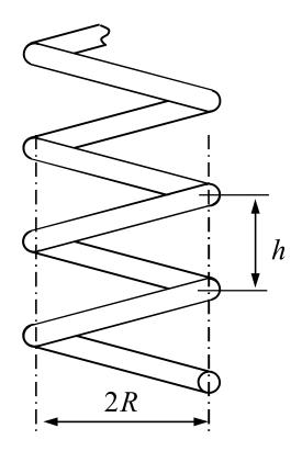
• A circular bar of radius R has zero twist. The basis vectors of (x, y, z) and (s, n, b) coordinate systems differ by rotation with respect to the normal direction to the plane of circle (z here). With distance s along the mid-curve and  $\phi = s / R$
