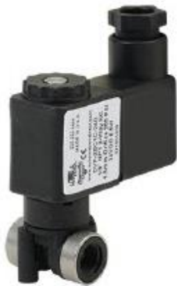
Figure 5B: 2-way, 2-position, normally closed direct-acting solenoid valve, spring return
