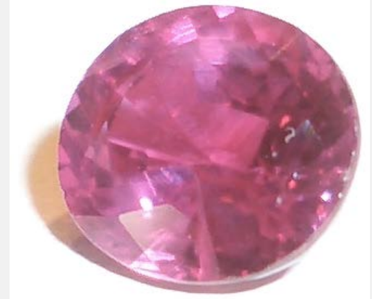
Ruby – Cr in \text{Al}_2\text{O}_3 matrix
