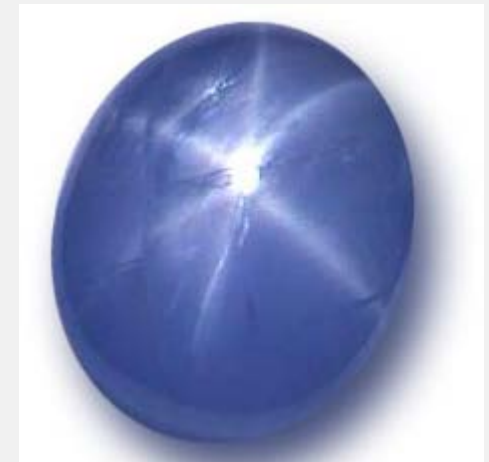
Sapphire – Ti and Fe in \text{Al}_2\text{O}_3
