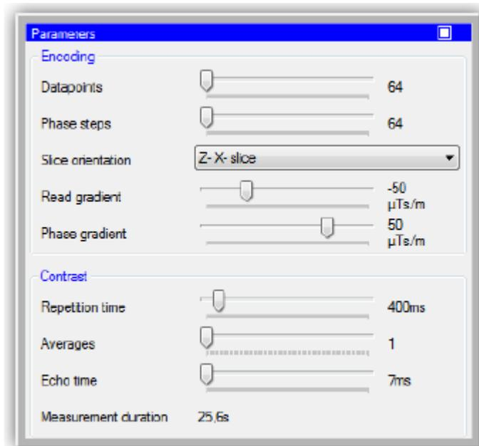
Figure 18: Parameters for experiment Spin Echo 2D
