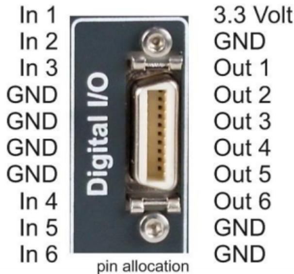
**Figure 3: Digital I/O – pin allocation**
