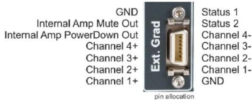
**Figure 4: External gradient amplifier – pin allocation**
