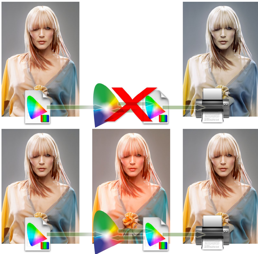
Figure 15 This illustration re-examines the problem encountered at the beginning of this chapter where the skin tones in the original image printed too blue. In the upper workflow no printer profile was used and the image data was sent directly to the printer with no adjustment made to the image data. In the lower example I show a profile color managed workflow. The profile created for this particular printer is used to convert the image data to that of the printer's color space before being sent to the printer. The (normally hidden) color shifting which occurs during the profile conversion process compensates by making the skin tone colors more red, but applies less color compensation to other colors. The result is an output that more closely matches the original. This is a simple illustration of the ICC-based color management system at work. All color can be managed this way in Photoshop, from capture source to the computer display and to the final print.
