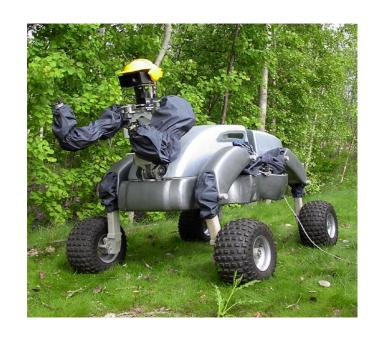
GPS-antenna Leg-control unit CCD-camera Navigation unit Main computer Laser pointer | Manipulator Body joint Engine
