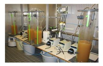
Sequencing Batch Reactors (SBRs) with operating volumes of 12 litres are operated in temperature-controlled chamber at  $17\pm1^{\circ}$ C ( $10\pm1^{\circ}$ C for Group 4). Feeding with synthetic wastewater during feeding sequence is done by peristaltic pumps with flow rate of 6 l/d. Fine bubble aerator is placed in the bottom of the reactors for constant aeration 2-3 l min<sup>-1</sup>). The SBR reactor is operated with an SRT of 12 days.
