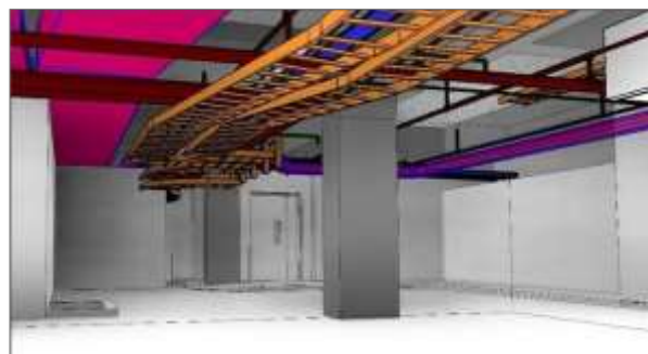
BIM model used for services coordination (Image source: China Construction (South Pacific))
