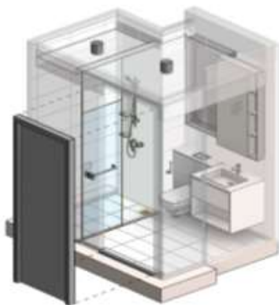
3D axonometric view of a bathroom extracted from the BIM model (Image source: China Construction (South Pacific))
