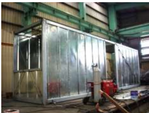
Mockup of a structural chassis for a PPVC module (Image source: P&T Consultants)
