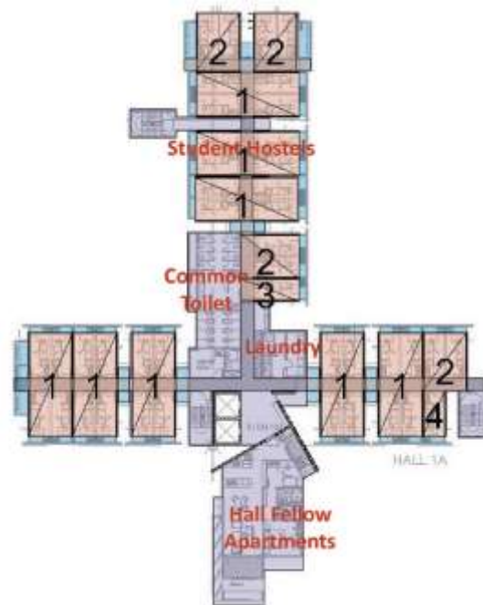
Determining a prefabrication approach based on a standardized building layout (Image source: P&T Consultants)
