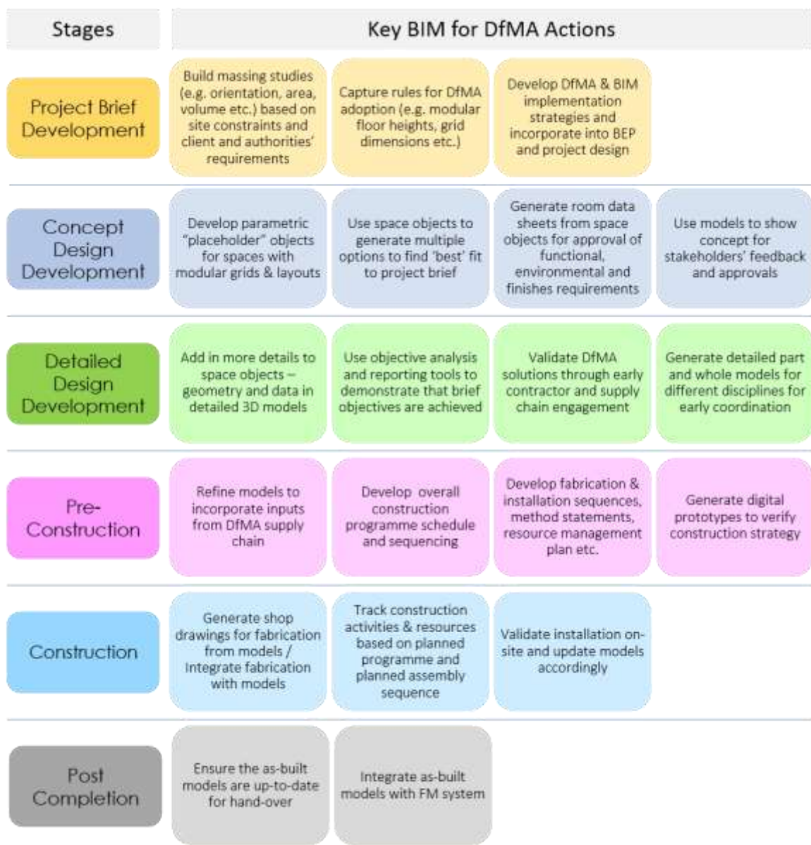
Key BIM actions for the DfMA approach at the various stages (Image source: BCA)
