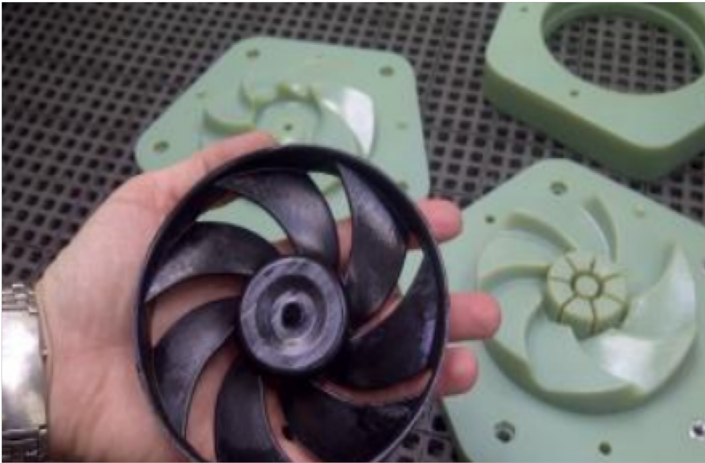
Injection molds printed with plastic
