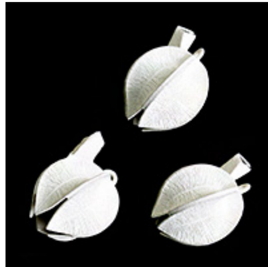
Printed wax masters for precision casting
