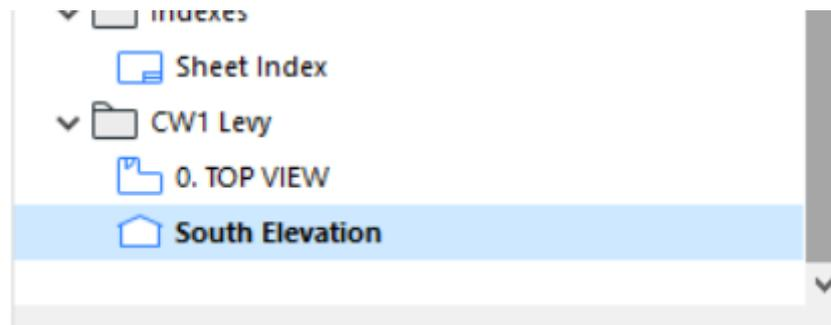
Go to "TOP VIEW". Select "section tool" from document tool group and place a section marker along x axis as shown below.
