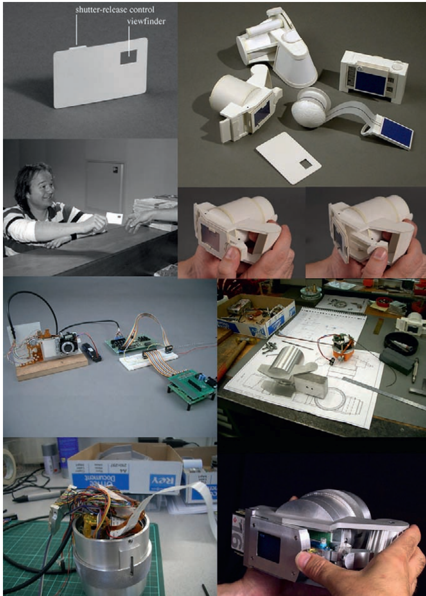
Figure 4.2 Joep Frens's approach to constructive design research. Building a rich interaction camera through mock-ups and prototypes. Top two left: details from a service scenario with a simple mock-up. Top three right: cardboard mock-ups from one camera variation. Below, clockwise from bottom left: fitting electronics into the cask, hacking existing technology; building a case, and final prototype of one camera. 8 (Pictures by Joep Frens.)
