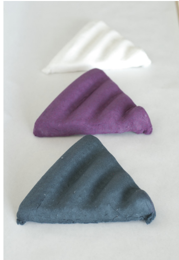
Figure 12.2 The gypsum mould for the new design (above), the second set of moulding tests (middle), and the prototypes made of dyed pulp with a triangular design (below).
