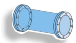
The pressure vessel (the thin walled tube) is loaded with an internal pressure  $p_o$  and a torsion moment  $M_t = \alpha p_0 t D^2$  resulting in a bi-axial membrane stress state. Assume a membrane stress state for the tube with a cylindrical symmetry.
