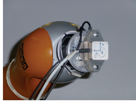
FIGURE 2: KUKA robot arm and the two independent IMU devices fixed to the tool. MicroStrain Inertia-Link is installed coaxially below SparkFun 6DOF Digital IMU which is inside the topmost aluminum enclosure.
