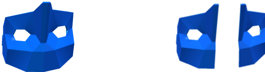
Figure 8. This mask is split in to two pieces to accommodate a smaller build volume (Principle 23)
