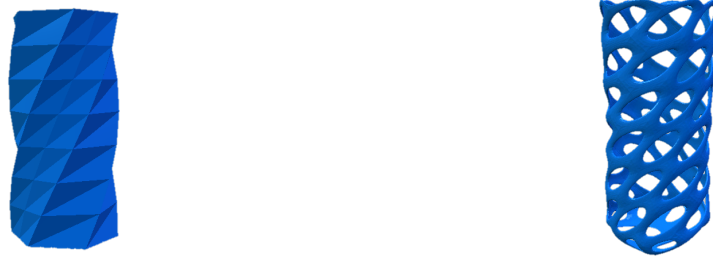
Figure 3. A vase's structure is replaced with a Vornoi structure to provide the same functionality with less material (Principle 5)
