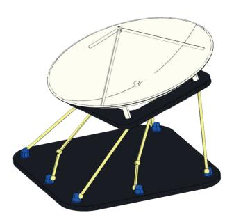
A structure made by six legs, pin-joints, and two platforms, which form the base and the roof, can be implemented in new, innovational solutions of antenna and solar panel systems, all designed by undergraduate students
