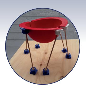
The Funnel Bowl is a system for pouring portions to a small container. When e.g. sand, or other similar substance, is poured into the upper two-piece bowl, the two halves will part because of the pressure of the sand and reveal a hole in the bottom. The hole allows the sand to flow to a smaller container. After the critical amount of sand has flown, the system will return to its original position.
